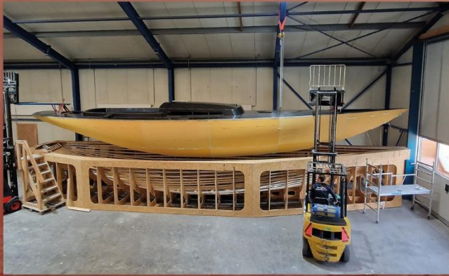
3D Core Kits™ for tool-less boatbuilding
