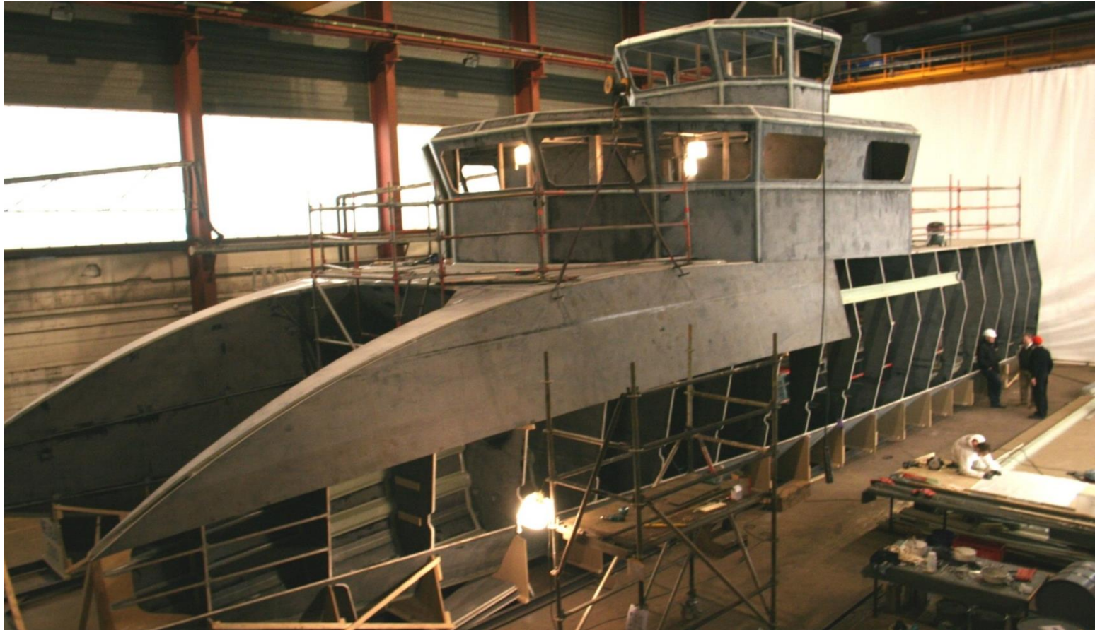
Bonding of frames, stringers, and outer skin of a 24m CTV
