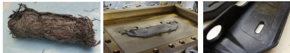
Compression molding material (BMC) from uncured prepreg residues/cut-offs
