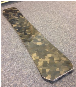
Uncured prepreg residues processed into chip laminate
