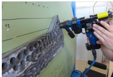
Uncured prepreg residues processed into drilling templates
