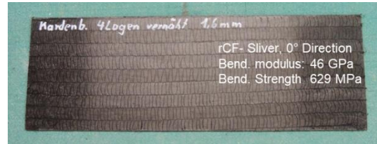
Highly aligned tows from short rCF for higher performance
