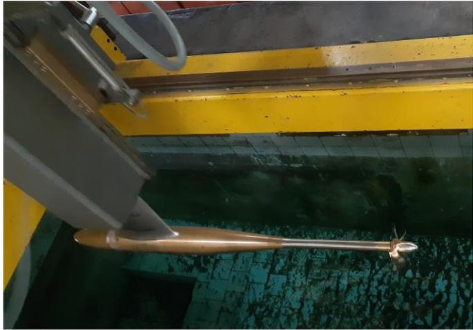
Metallic propeller (rigid) : optimal for **one operating condition**
