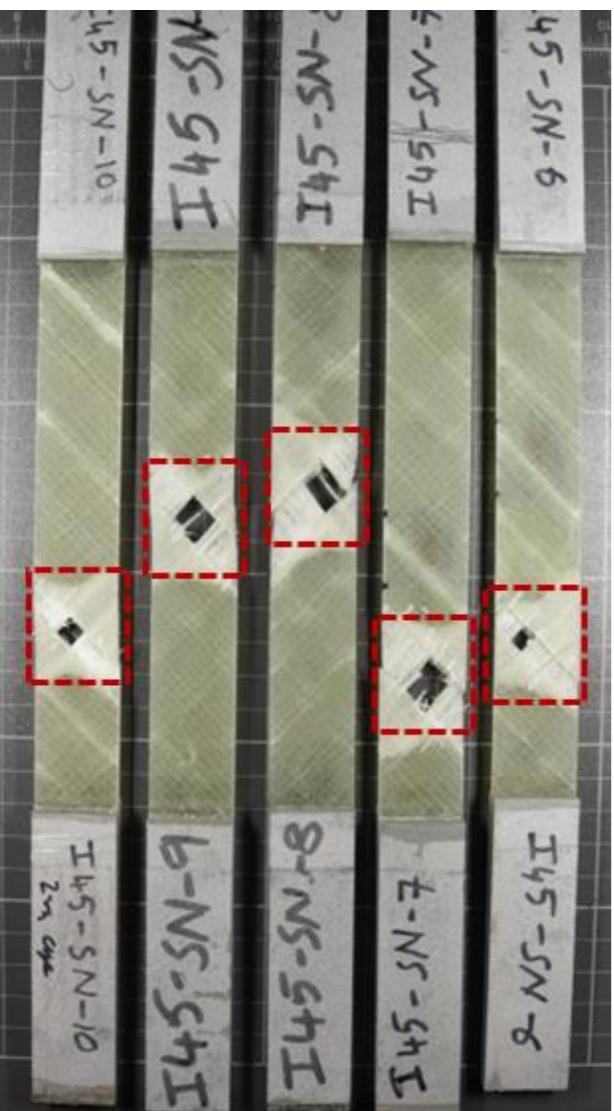
Location of final failure indicated on the specimens.
