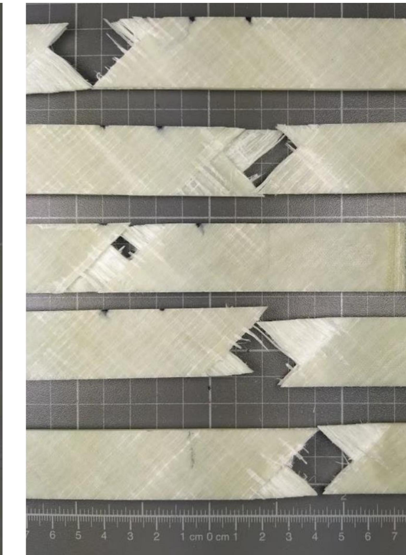
Failed coupons: [ $\pm 45^\circ$ ] Glass/Thermoplastic
