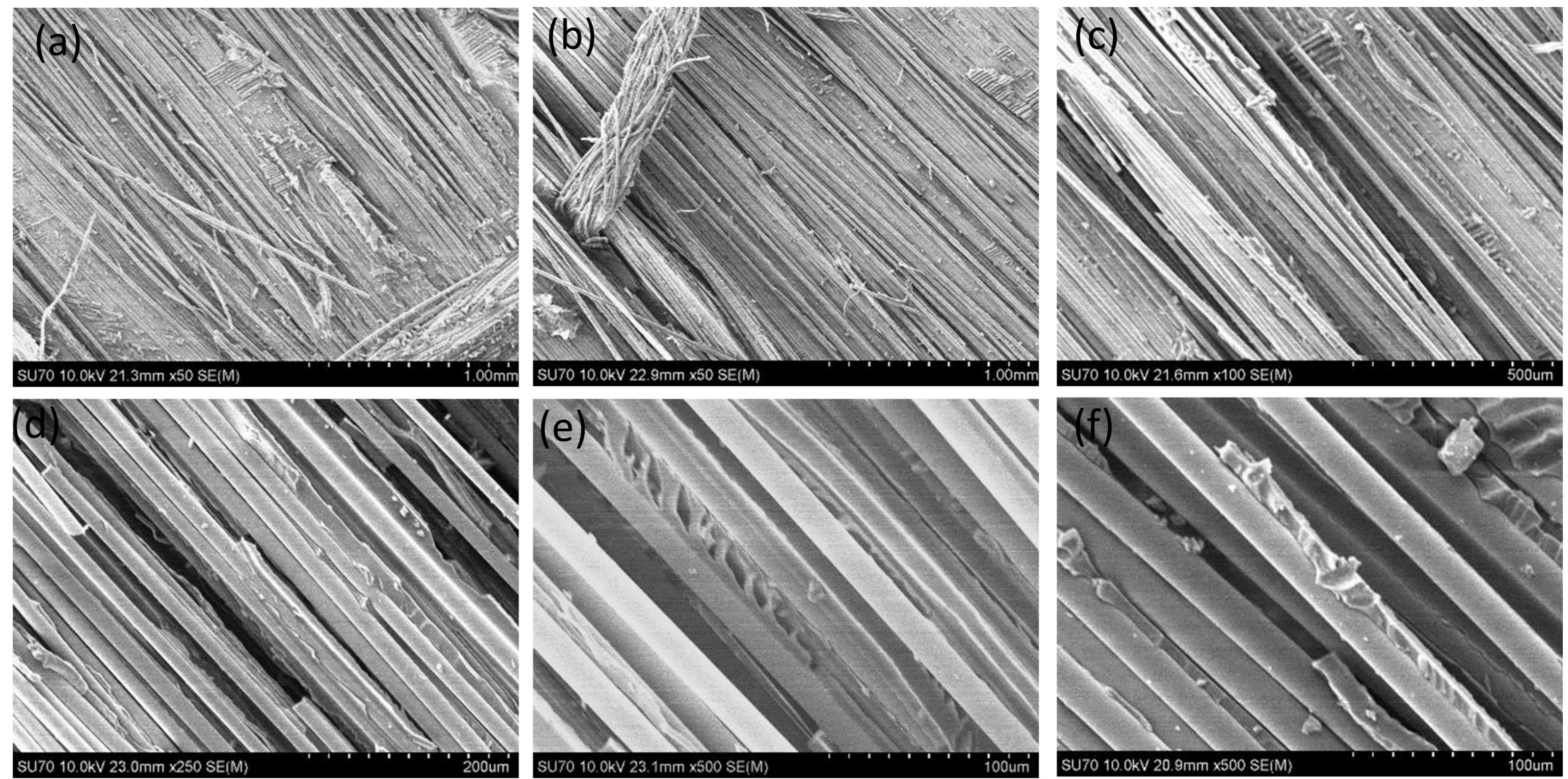
Low-cycle fatigue tested GF/Elium 45° specimen
