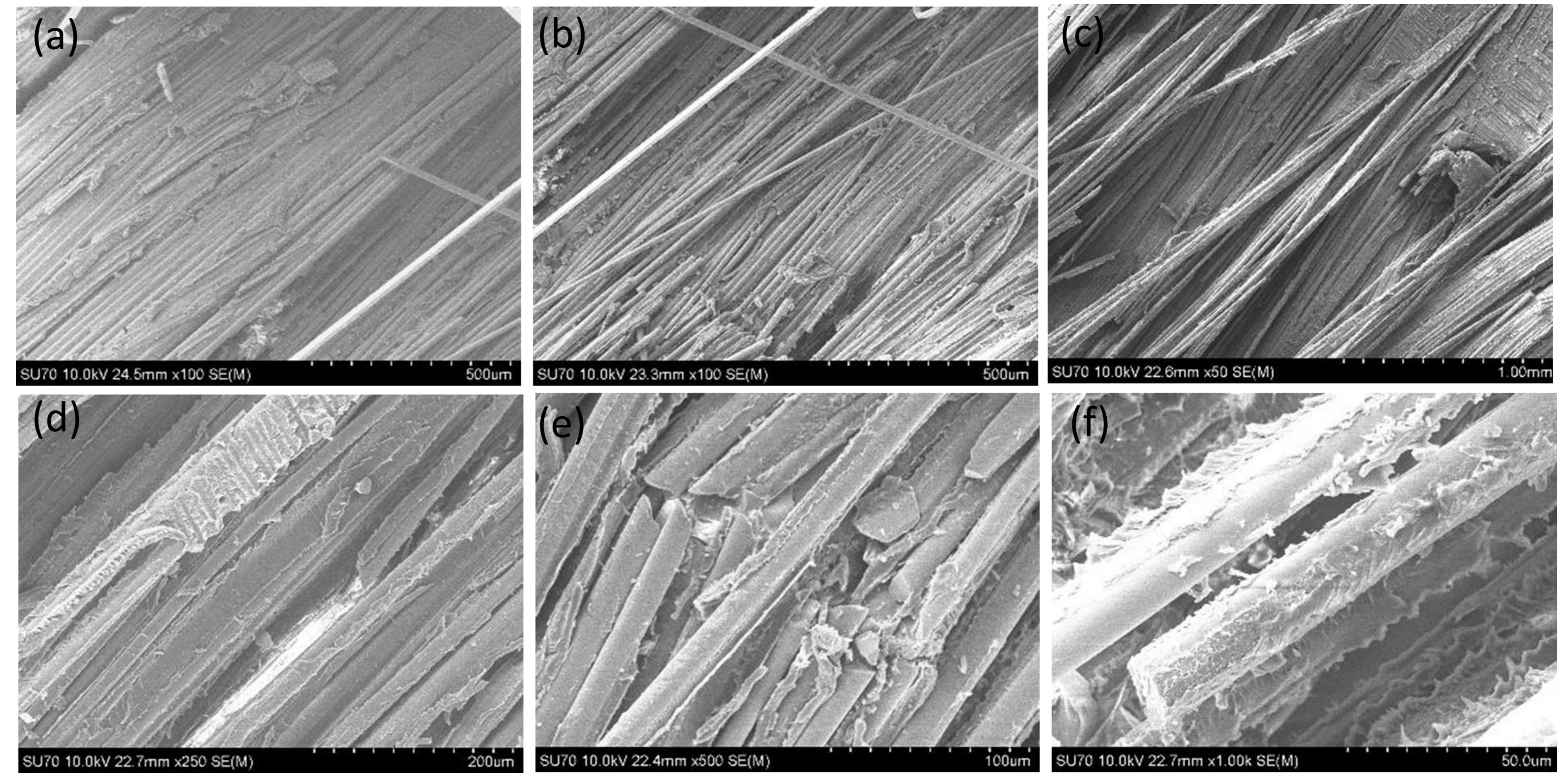
High-cycle fatigue tested GF/Infugreen 45° specimen
