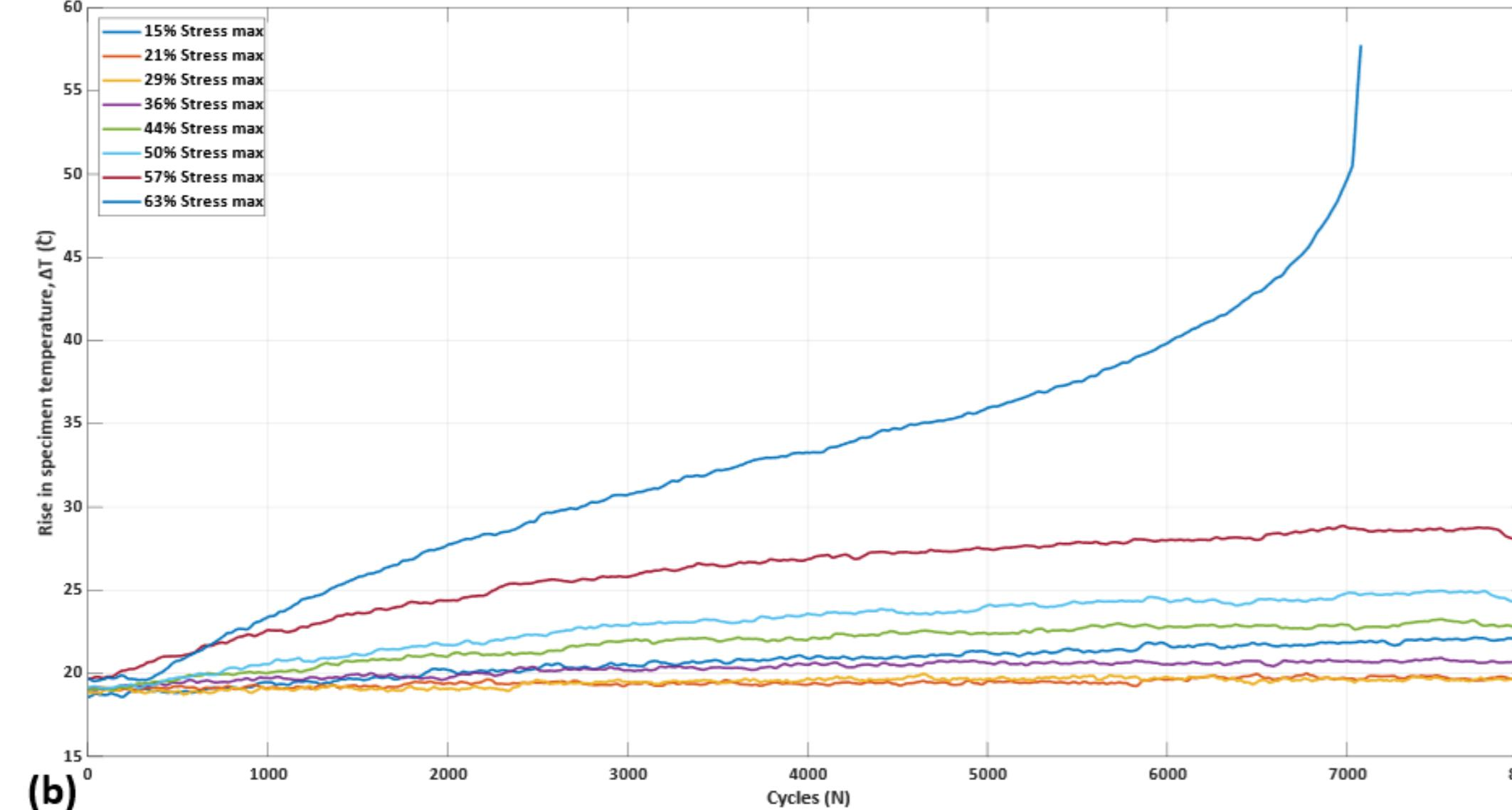
Evolution of (a) Damage and (b) Temperature in  $\pm 45^\circ$  GF/THERMOSET.
