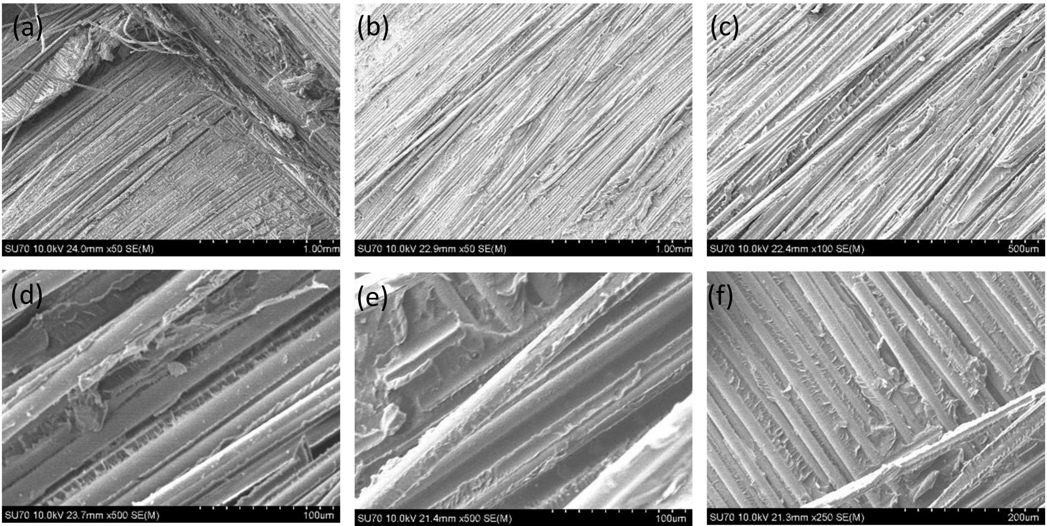
Low-cycle fatigue tested GF/Infugreen 45° specimen
