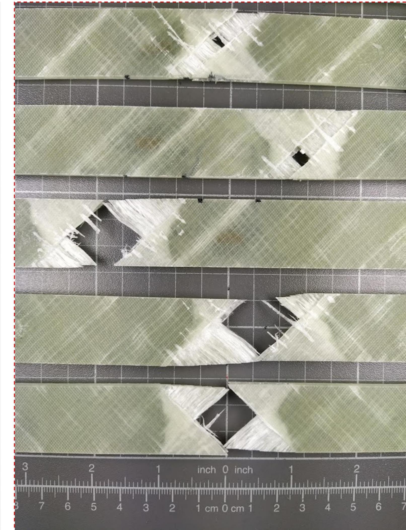
**Failed coupons: [ $\pm 45^\circ$ ] Glass/THERMOSET**
