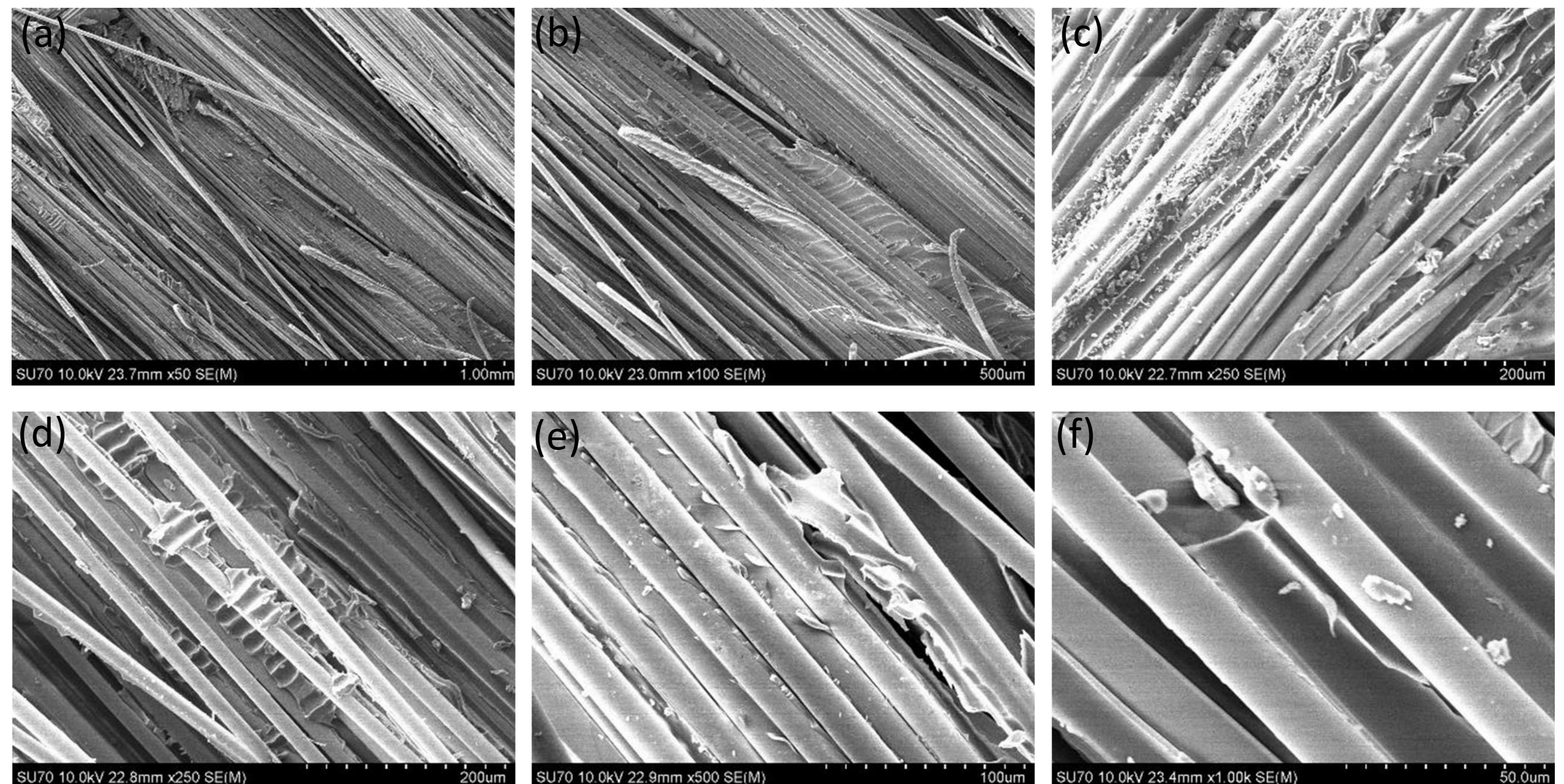
High-cycle fatigue tested GF/Elium 45° specimen
