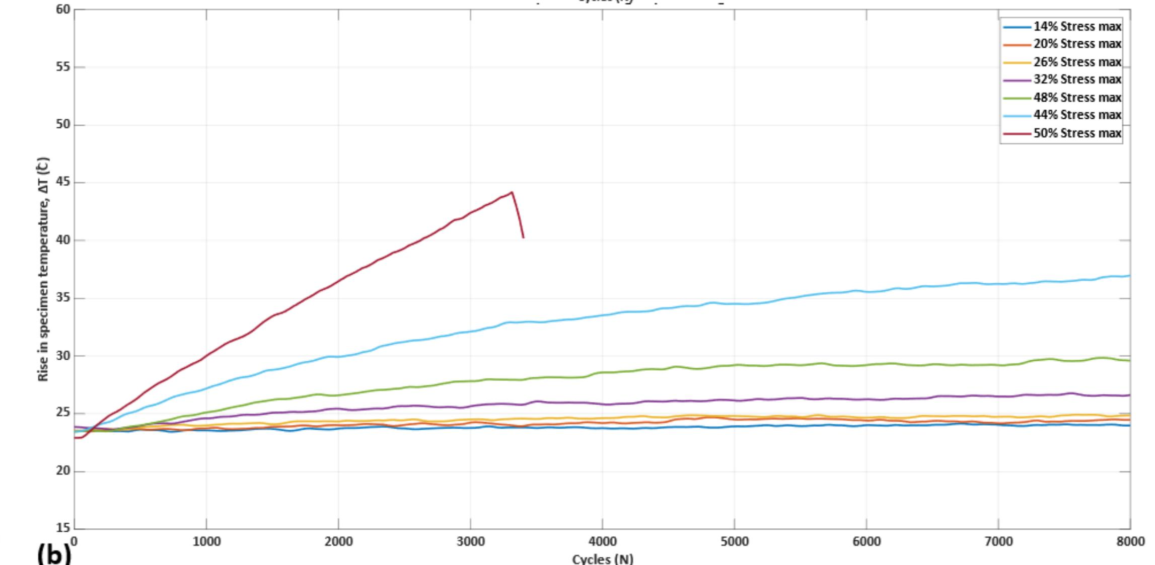
Evolution of (a) Damage and (b) Temperature in  $\pm 45^\circ$  GF/Thermoplastic.
