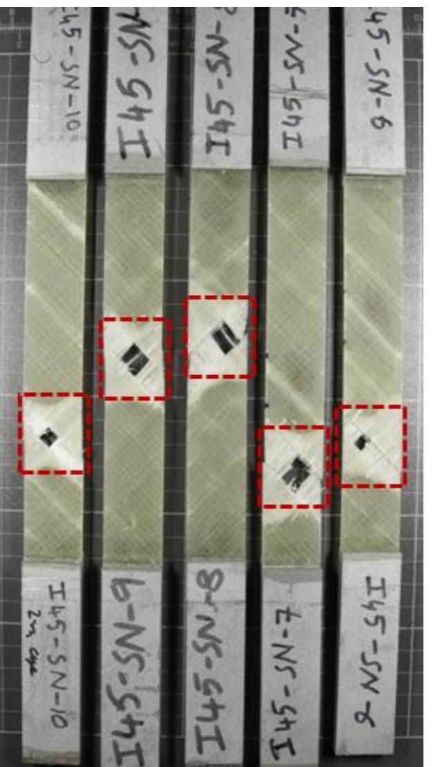
Location of final failure indicated on the specimens.
