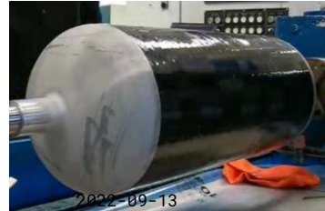
CF "liner" with dome ends for final winding
