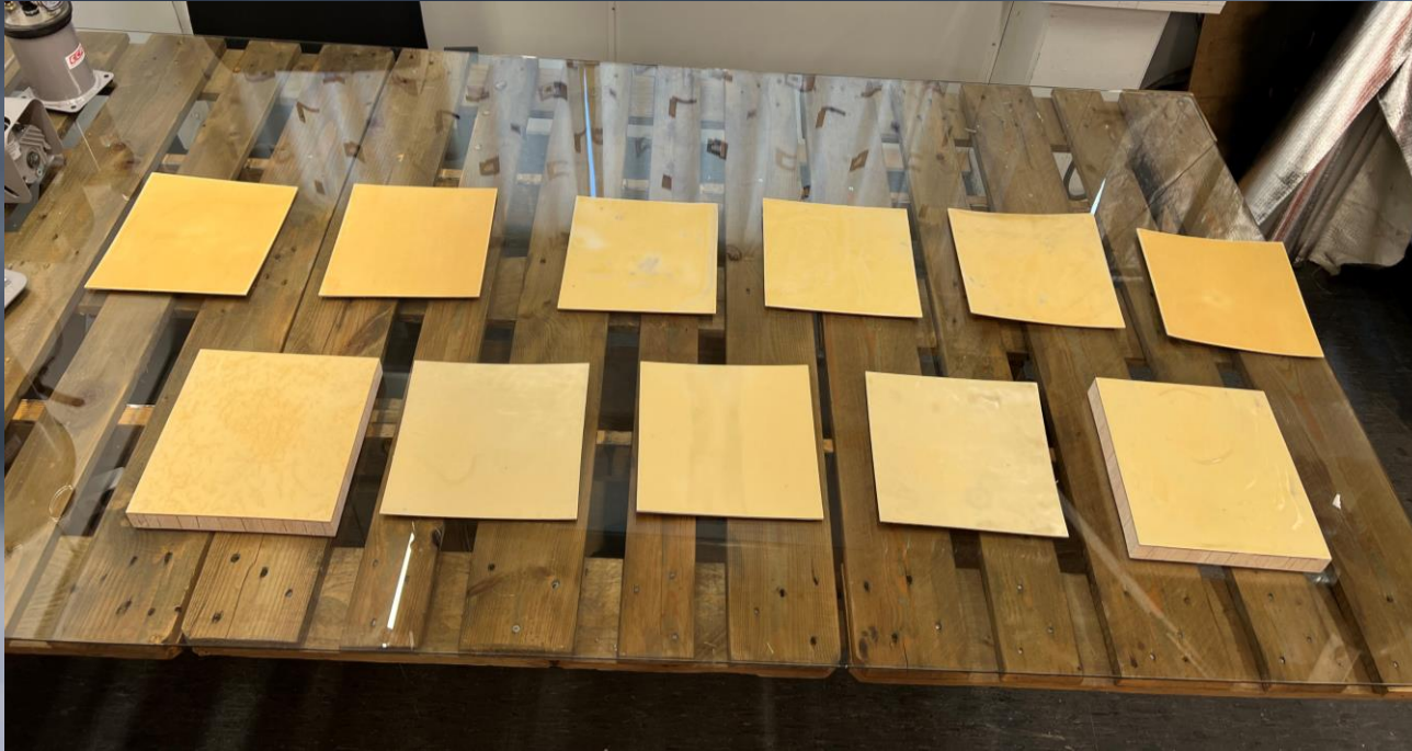
11 layups prepared for cone calorimeter testing.
