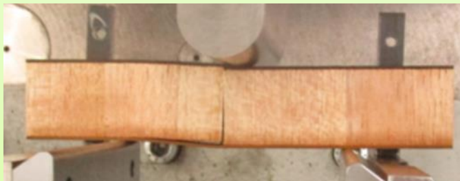
PFA prepreg for Cabin floor at Chantiers de l'Atlantique (I8)
