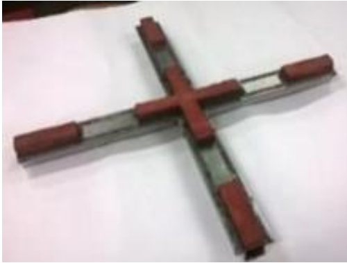
Metal profiles equipped with Sylomer®-strips
