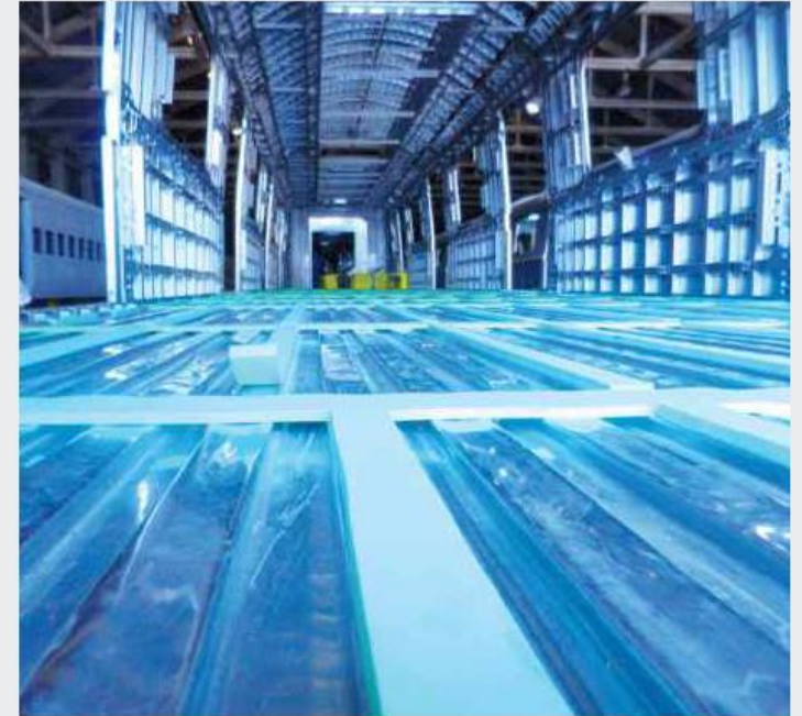
Sylomer® decoupling in underground carriage
