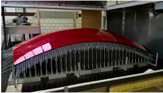
Figure 10: The adaptive mould at Curve Works
