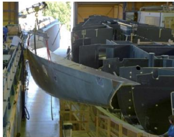
Figure 6: Hull construction of the Pink Gin VI [5]
