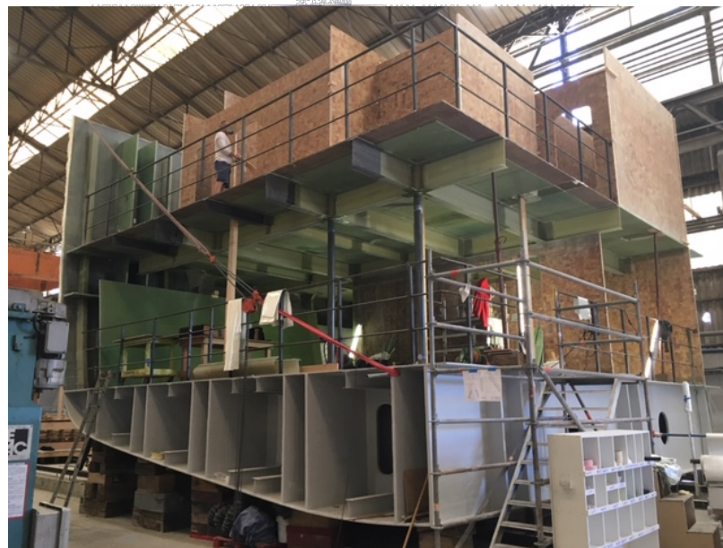
Demonstrator: Engine room and other above accommodation spaces. 11m x 11m x 8.6m
