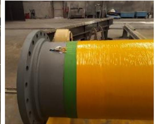
Fe coating FBG sensor for marine corrosion
