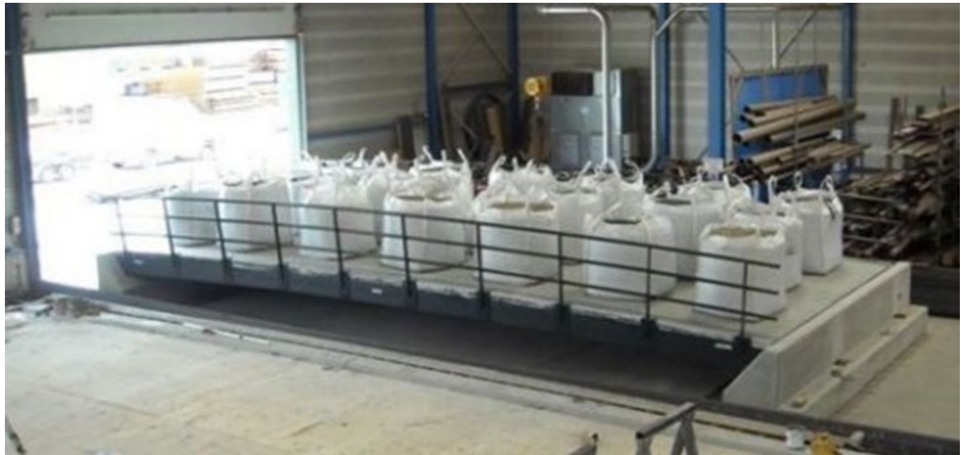
Full-scale test Lotharingen bridge, Utrecht. Lightweight Structures and Damsteegt
