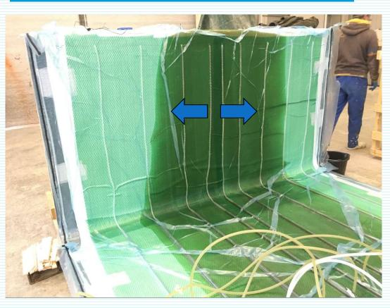
Flow on surface and through the thickness infusion
