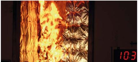
CSC components are seen here being fire tested
