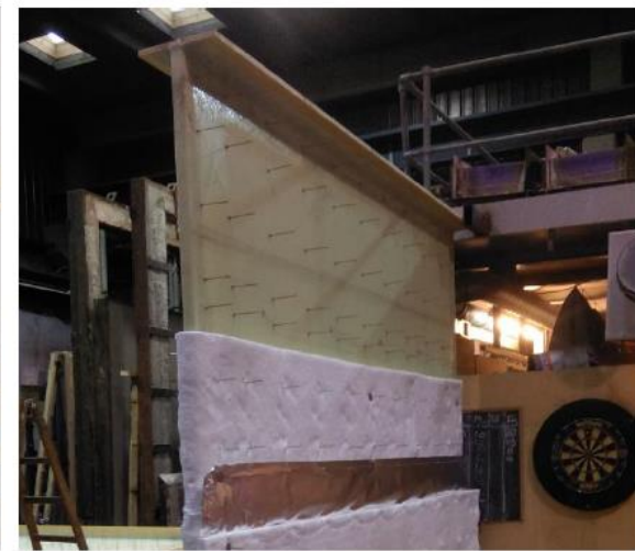
1 x XE905 Biaxial E-glass +/-45 1 x XE905 Biaxial E-glass +/-45 40 mm Divinycell P100 1 x XE905 Biaxial E-glass -/+45 1 x XE905 Biaxial E-glass -/+ 45
