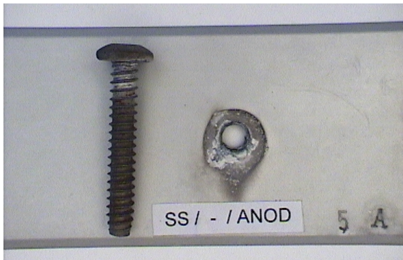
c) Stainless steel screw / anodised extrusion
