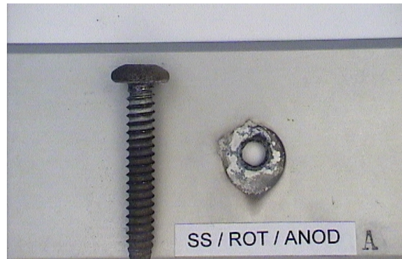
d) Stainless steel screw / Rotalyt / anodised extrusion
