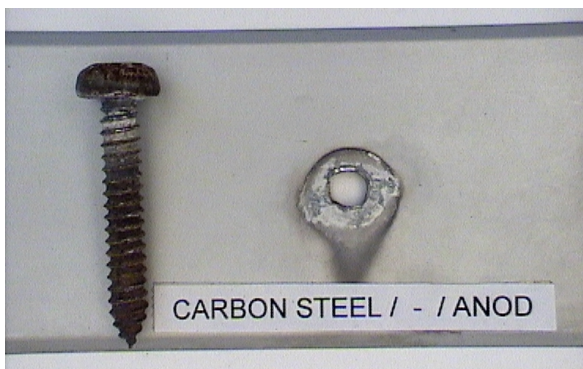
g) Carbon steel screw / anodised extrusion
