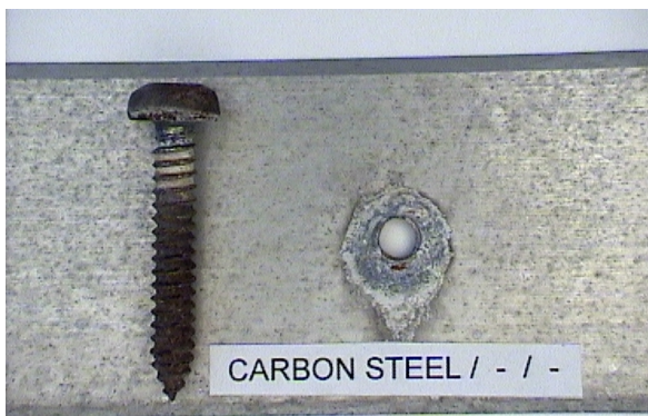
e) Carbon steel screw / no surface treated extrusion
