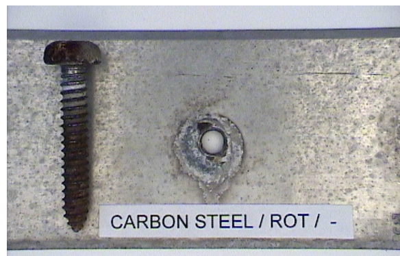
f) Carbon steel screw / Rotalyt / no surface treated extrusion
