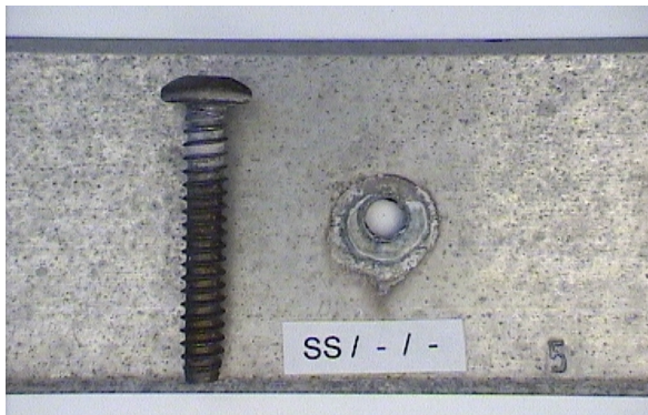
a) Stainless steel screw / no surface treated extrusion
