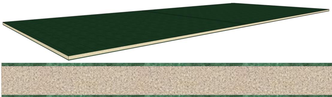
Figure 2.4. Illustration of an FRP composite panel (top) and a close-up on the lightweight core and the rigid and strong fibre reinforced laminates (bottom).
