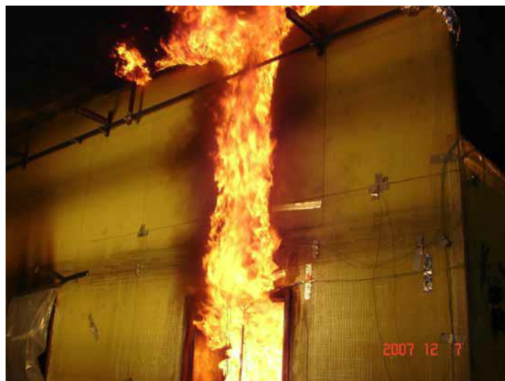
Figure 4.6. FRP composite surface which has been exposed to flames from a fully developed fire through a window opening for 4.5-5 minutes.
