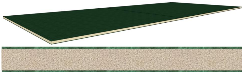
Figure C1. Illustration of an FRP composite panel (top) and a close-up on the lightweight core and the rigid and strong fibre reinforced laminates (bottom).
