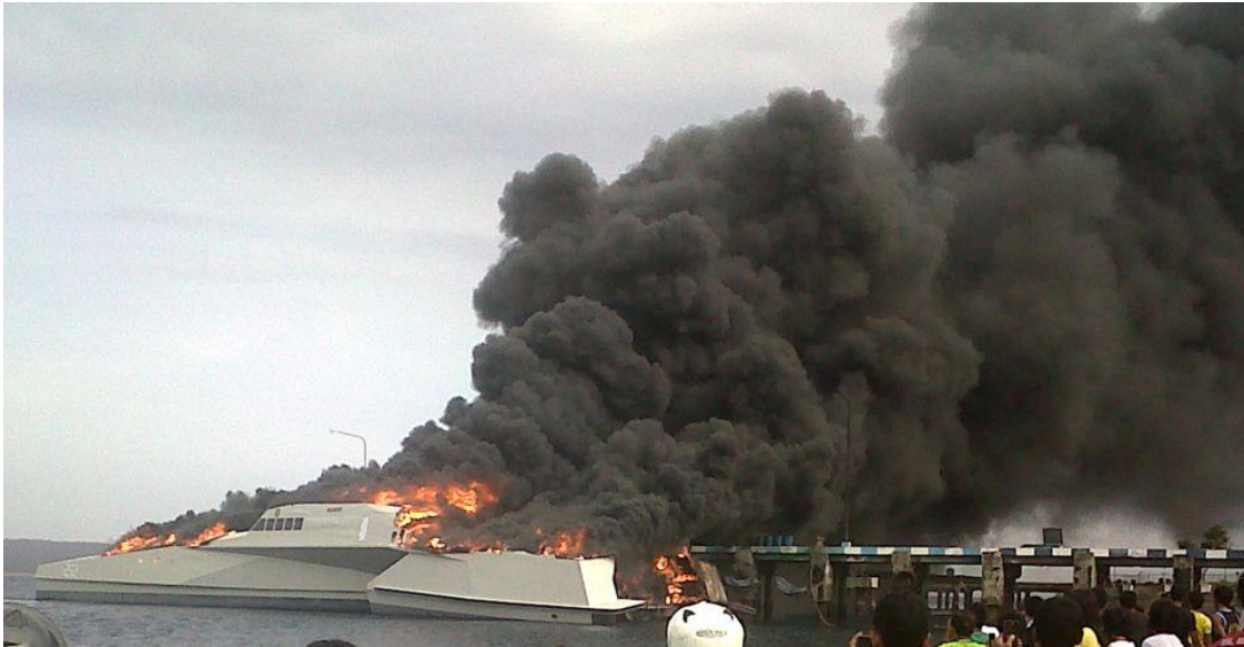
Figure 4.8. The Indonesian navy ship Kri Klewang had unprotected FRP composite surfaces on exteriors where a catastrophic fire established. (photo: skalanews.com)
