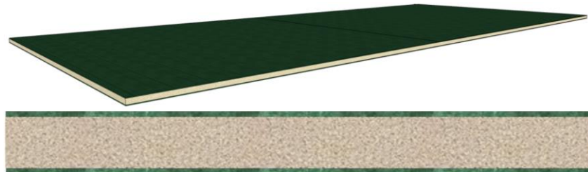
Figure C1. Illustration of an FRP composite panel (top) and a close-up on the lightweight core and the rigid and strong fibre reinforced laminates (bottom).
