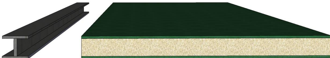
Figure C2. Illustration of how the lightweight core works as a prolate stiffener in order to provide the FRP composite panel with a distribution of loads similar to an “I-beam”.
