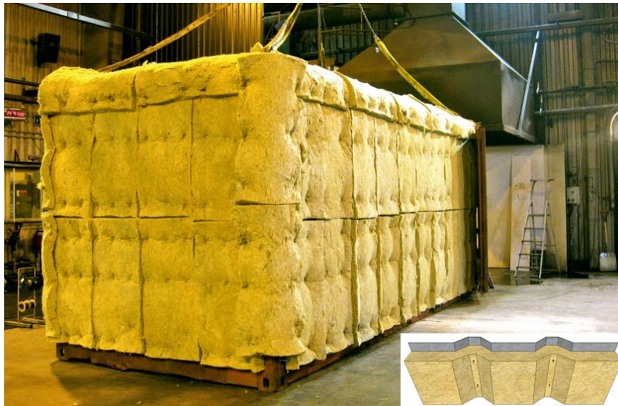
Figure 4.8. The insulated steel container, ready to be used in the experiments.
