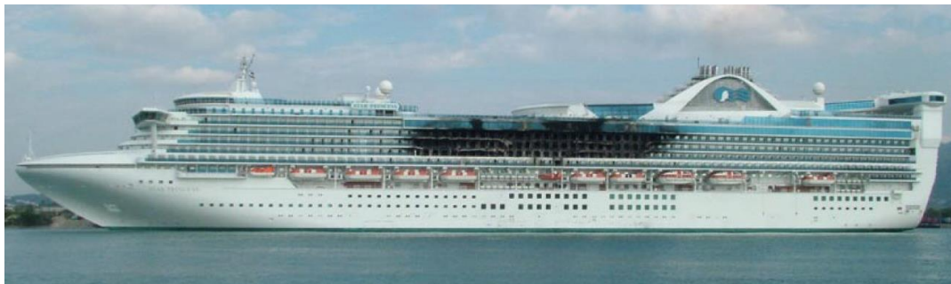
Figure 4.14. Extent of damage on port side of the Star Princess after outboard fire spread [25].
