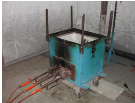
Figure 16 Small-scale furnace for structural resistance tests.
