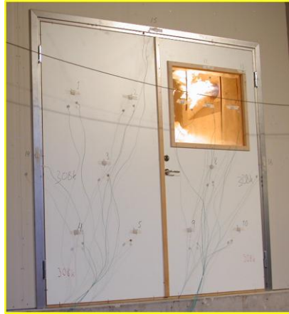
Figure 15 Insulation test of a door where thermocouples measure the backside temperature during the heat exposure.
