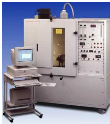
Figure 12 Smoke box equipment.
