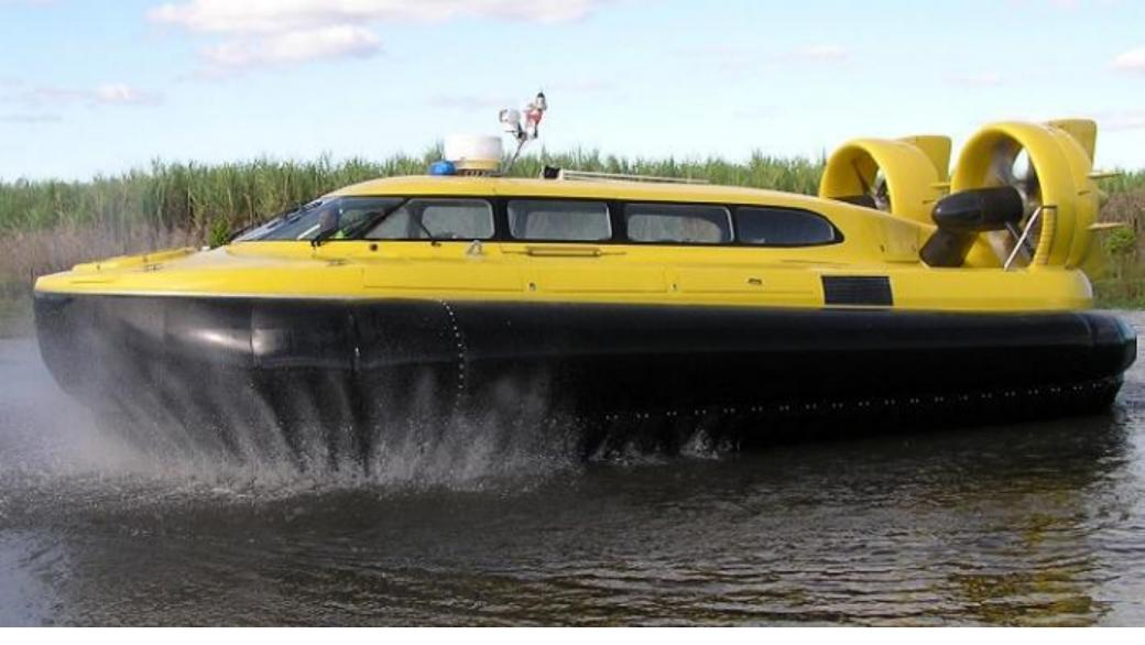
The Pioneer Mk3 hovercraft built at the China factory has capacity of 25 passengers or 2.5 tonnes payload + 1 crew. The air-conditioned cabin provides comfortable seating and good visibility for the passengers and crew. The Pioneer Mk3 is powered by two Steyr diesel engines of 190kW each and will cruise comfortably at 25 to 30 knots with higher speed on demand.
