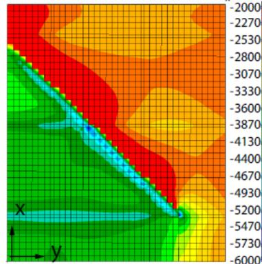
Longitudinal normal strain,  $\epsilon_x$  [ $\mu\text{m}/\text{m}$ ]
