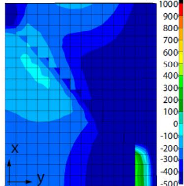
Transverse normal strain,  $\epsilon_y$  [ $\mu\text{m}/\text{m}$ ]
