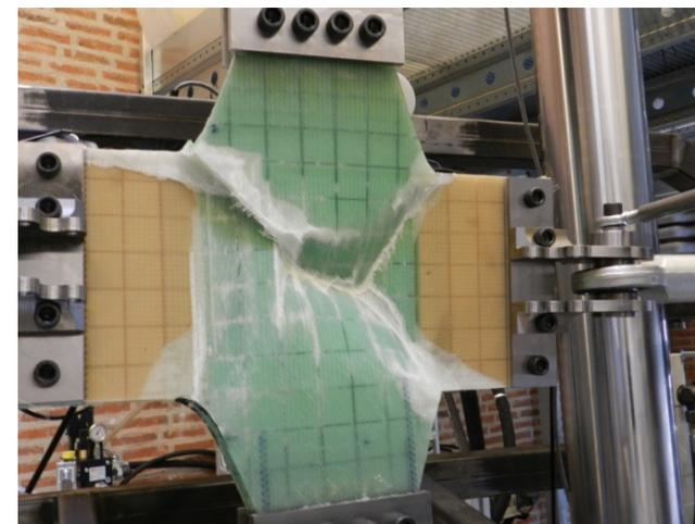
Post mortem images showing through-thickness (z direction) cracks in the longitudinal resin bridge when subjected to the **multi-axial tension load case**.
