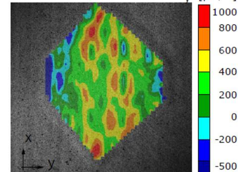
Global and local FE model predictions vs. DIC measurements for the *multiaxial compression case* at  $P_L = -60$  kN.
