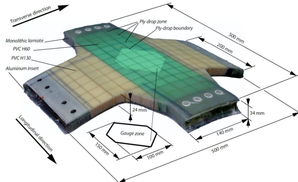
Biaxial compression loading - cyclic fatigue
