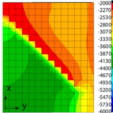
Longitudinal normal strain,  $\epsilon_x$  [ $\mu\text{m}/\text{m}$ ]
