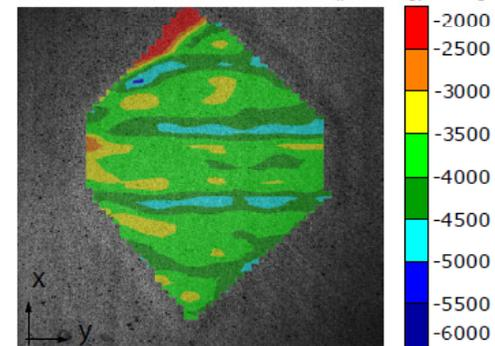
Transverse normal strain,  $\epsilon_y$  [ $\mu\text{m}/\text{m}$ ]
