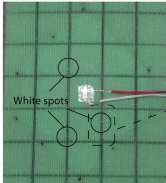
Through-thickness view of a longitudinal resin bridge
