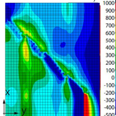
Transverse normal strain,  $\epsilon_y$  [ $\mu\text{m}/\text{m}$ ]
