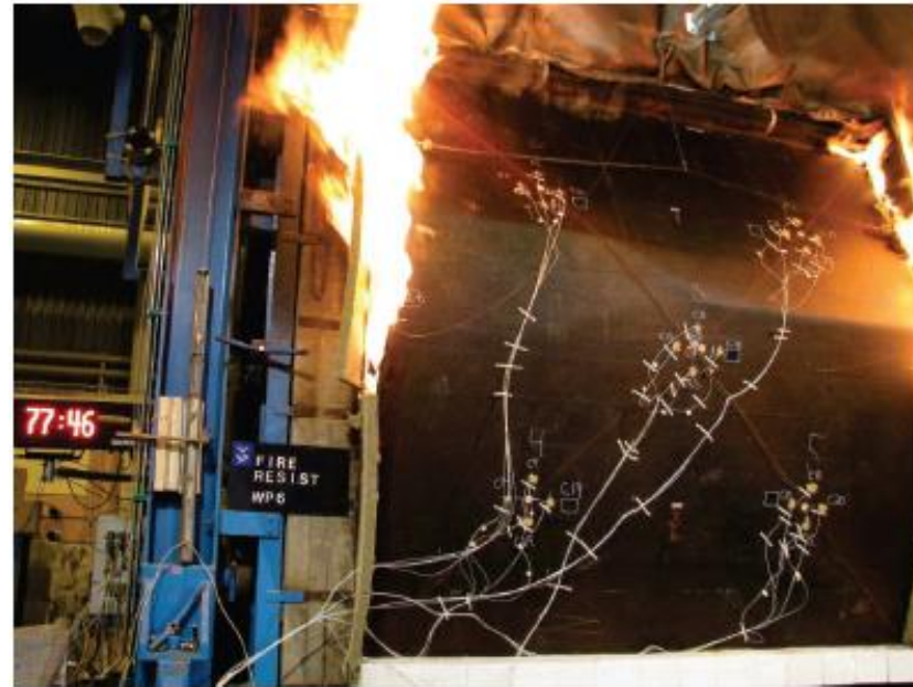
Failure @ 7kN/m load after 77min
