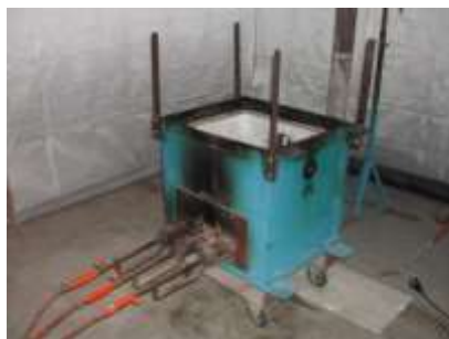
Figure 14: Small-scale furnace for structural resistance tests
