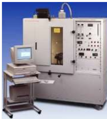
Figure 10: Smoke box equipment
