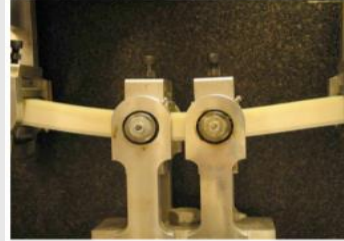
Figure 1. Four-point bending rig
